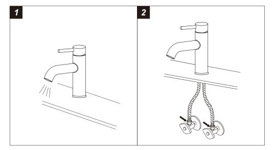
1. Turn the faucet handle all the way on, turn on hot and cold water supply and flush water lines for one minute. 2. Check all connections at arrows for leaks, re-tighten it if necessary.
