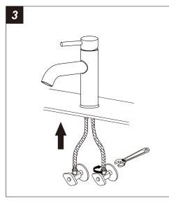
3.Connect the flexible hoses to water supply valve (not included) and copper tubes, and tighten it with adjustable wrench. DON'T OVER TIGHTEN!
